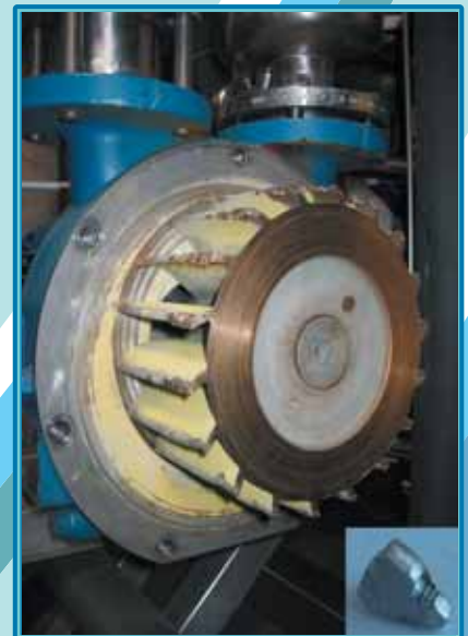
Pump Failure Resulting From a Screw Which had Worked Loose
